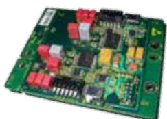
The PPM Phono Preamp Module can be used with both MM and MC cartridges and allows custom loading. It is an option available for the Sigma SSP and CP-800 preamp/processors.
