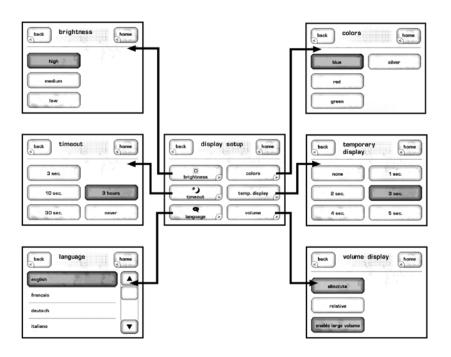
The **display setup** menu allows you to define your preferences for three aspects of the CDP-300's LCD display: the **brightness** of the backlighting, the **timeout** of the backlighting, and the **language** used.
