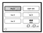
The **operational menu** provides easy access to the most basic functions of the preamplifier: **input selection** and **tape monitor**. It also provides both a numeric and a graphic depiction of the current **volume** setting.
