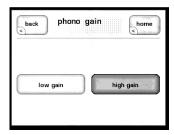
The **phono gain** menu is only active if the optional **phono module** is installed; otherwise it is grayed out. When it is installed, the CP-500 will automatically recognize it, rename the **line 1** input to **phono**, and activate the input on the main menu.
