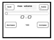
The **max volume** screen allows you to establish a maximum volume setting for your system. This scale runs from 0 to 100, with 100 indicating that you do not want any artificial limit placed on the maximum gain your preamplifier can provide.
