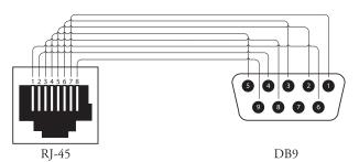
Remarks: The Cat 5 cable and connector that is used for the adaptor and plugs into the rear panel RJ-45 port must use pin-to-pin wiring.
