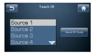
The Teach IR page displays a scrolling list of all the available IR codes in the Sigma 2200i. Simply scroll to the command you want your macro-capable remote to learn and touch the **Send IR Code** button. The Sigma 2200i continuously sends that command code via the front panel - as long as the button is pressed – until your third-party remote control has learned it.
