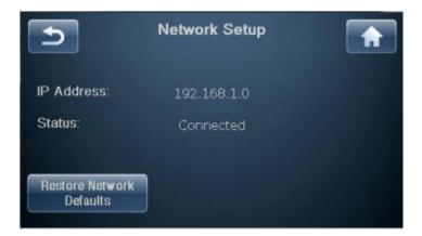
The Sigma 2200i includes a built-in web interface that can be used to configure the system name, Network settings and update its software. To access the interface, type the IP address displayed on the Network Setup page in the URL line of your browser (e.g. 192.168.1.0) and hit return. Alternately if you are using Safari on the Mac, you can "Show All Bookmarks" (See: Bookmarks menu) and click on Bonjour and double click on your Sigma 2200i device listed in the Webpage's folder.
