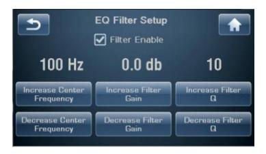
You do not need to have all or even any filters enabled for a given channel. The installer need only make the adjustments to the channel(s) necessary to correct for the room's interaction. We encourage you to consult with your authorized Classé dealer to properly calibrate the Parametric EQ function.
