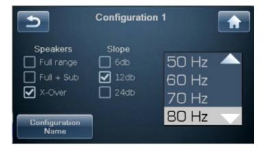
If you also want to High-Pass Filter the L&R Speaker outputs, check the X-Over box. The crossover will pass the higher frequencies and correctly direct the low frequencies to the subwoofer based on your frequency and slope settings.
